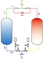
The expansion from operating pressure to atmospheric pressure will allows the small stream of dried air to remove the moisture that is adsorbed by the desiccant. Pressurisation will take place after vessel B is completely regenerated. The dryer cycle will then switch over and repeat the whole cycle.
